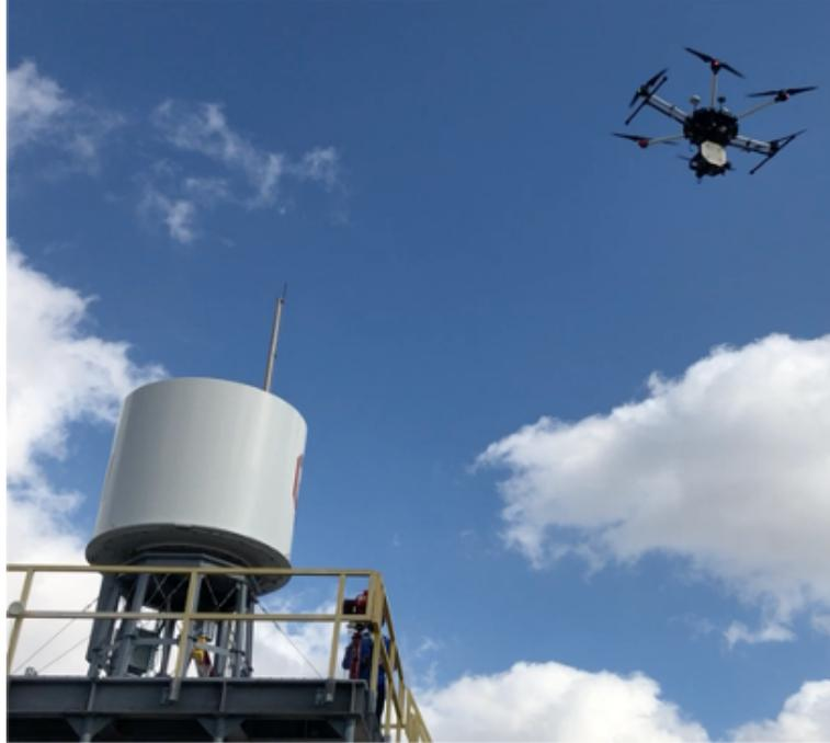
Figure 6.1: CPPAR system mounted on the rooftop of the Radar Innovations Laboratory (RIL), and the UAV-based system during a mission.
