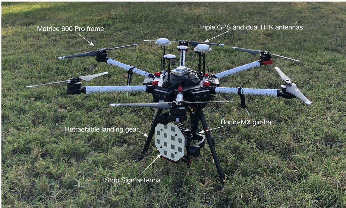
Figure 5.5: The DJI Matrice 600 Pro platform with the Ronin-MX gimbal and the SS probe antenna, with triple GPS sensors for redundancy during flight, and dual RTK antennas for increased positioning accuracy.
