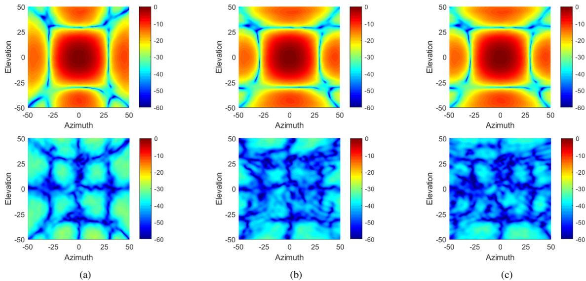
Fig. 19: Measured polarimetric 4x4 planar phased array radiation patterns with V-polarization at broadside; co- and cross-polarization magnitude in dB according to (a) Ludwig 2-I, (b) Ludwig 2-II (second row), and (c) Ludwig 3.
