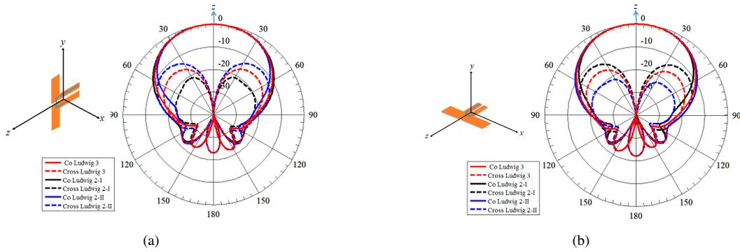
Fig. 9: Numerical simulations of co- and cross-polarization radiation patterns according to Ludwig's definitions in the  $D$ -plane of a printed dipole antenna polarized in (a) the  $y$ -direction and (b) the  $x$ -direction.
