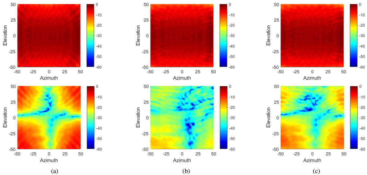
Fig. 17: Measured radiation patterns of the unit cell antenna at 3 GHz with V-polarization; co- and cross-polarization magnitude in dB according to (a) Ludwig 2-I, (b) Ludwig 2-II (second row), and (c) Ludwig 3.
