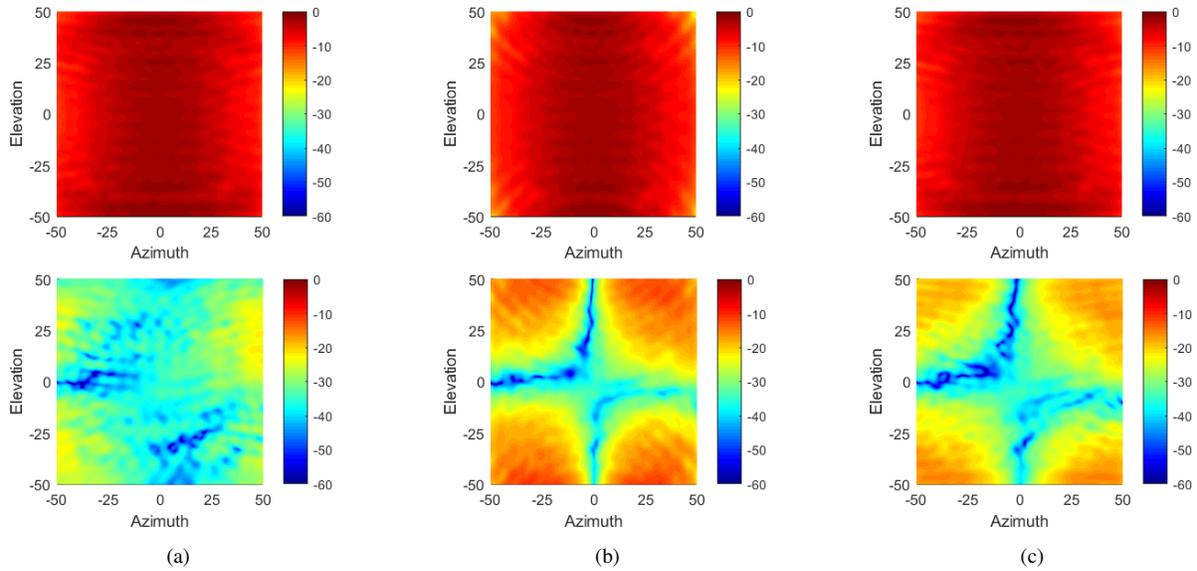
Fig. 16: Measured radiation patterns of the unit cell antenna at 3 GHz with H-polarization; co- and cross-polarization magnitude in dB according to (a) Ludwig 2-I, (b) Ludwig 2-II (second row), and (c) Ludwig 3.
