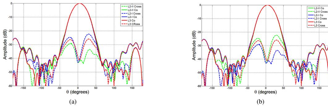
Fig. 13: Measured antenna patterns of a pyramidal horn antenna using Ludwig’s definitions when the current source is polarized in (a) the  $x$ -direction and (b) the  $y$ -direction.
