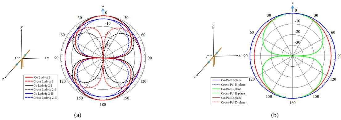
Fig. 6: Numerical simulations of co- and cross-polarization radiation patterns in the  $D$ -plane of a  $\lambda/2$  electric dipole antenna polarized in the  $z$ -direction according to (a) Ludwig’s definitions (improper definition) and (b) proper definition ( $E_\theta$  and  $E_\phi$ ).
