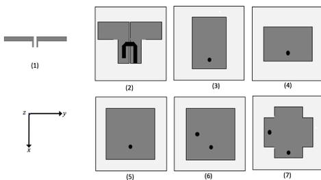
Fig. 14: Geometry of proposed antennas: wire dipole (1), printed dipole (2), narrow-side-fed rectangular patch (3), wide-side-fed rectangular patch (4), single-polarized square patch (5), dual-polarized square patch (6), and dual-polarized crossed-patch antenna (7).
