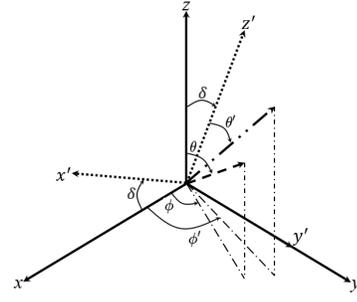
Fig. 4: Spherical coordinate system for a reference and tilted system shown in black solid and dotted, respectively.
