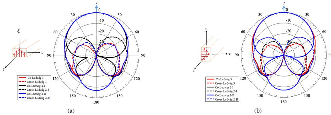
Fig. 8: Numerical simulations of co- and cross-polarization radiation patterns according to Ludwig's definitions in the  $D$ -plane of an open-ended rectangular waveguide antenna polarized in (a) the  $y$ -direction and (b) the  $x$ -direction.
