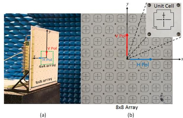
Fig. 15: Near-field chamber setup for electronic scanned radiation patterns of an array 4x4 elements embedded in an array of 8x8 elements at 3 GHz. (b) Top-view of the 8x8 antenna array and unit cell element [16].
