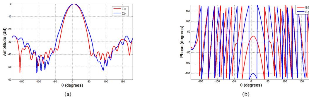
Fig. 12: Measured  $E_\theta$  and  $E_\phi$  components in the  $D$ -plane of a pyramidal horn antenna (a) amplitude (dB) and (b) phase ( $^\circ$ ).
