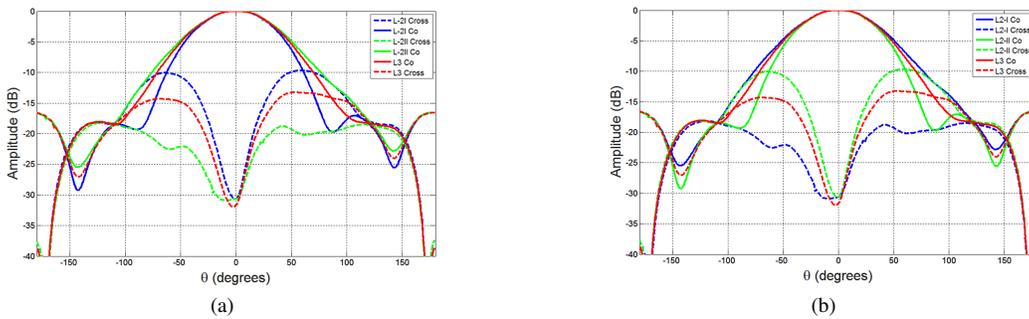
Fig. 11: Measured antenna patterns of a microstrip patch antenna using Ludwig's definitions when the current source is polarized in (a) the  $x$ -direction and (b) the  $y$ -direction.
