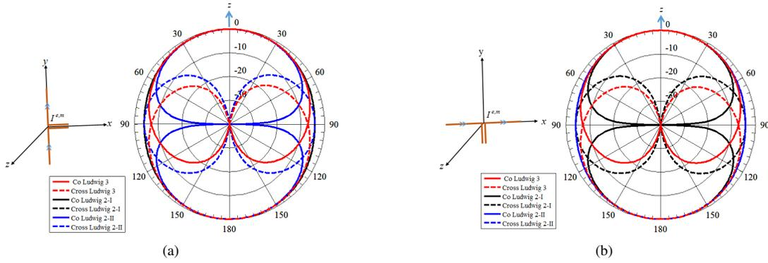
Fig. 5: Numerical simulations of co- and cross-polarization radiation patterns according to Ludwig’s definitions in the  $D$ -plane of a  $\lambda/2$  electric dipole antenna polarized in (a) the  $y$ -direction and (b) the  $x$ -direction.
