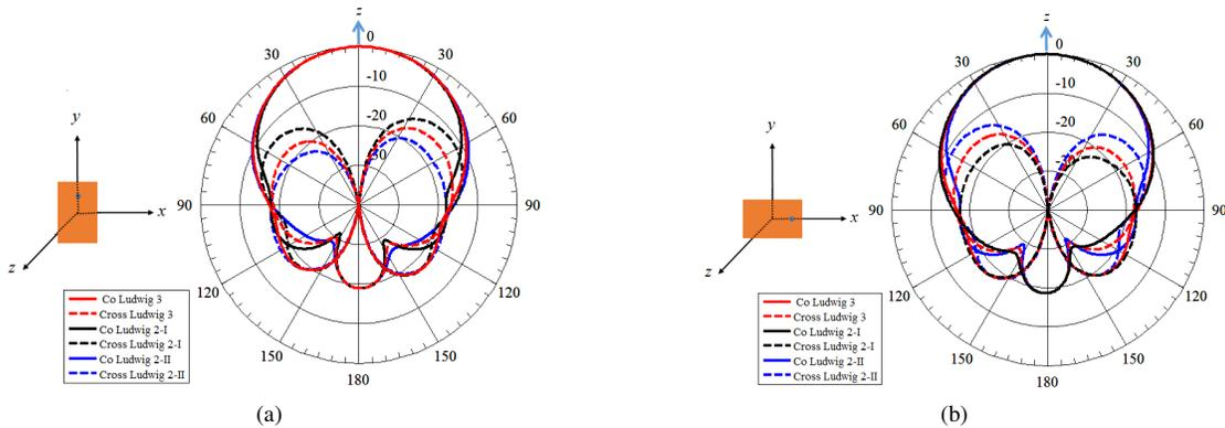
Fig. 7: Numerical simulations of co- and cross-polarization radiation patterns according to Ludwig definitions in the  $D$ -plane of a rectangular microstrip patch antenna polarized in (a) the  $y$ -direction and (b) the  $x$ -direction.
