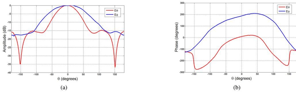
Fig. 10: Measured  $E_\theta$  and  $E_\phi$  components in the  $D$ -plane of a microstrip patch antenna (a) amplitude (dB) and (b) phase ( $^\circ$ ).
