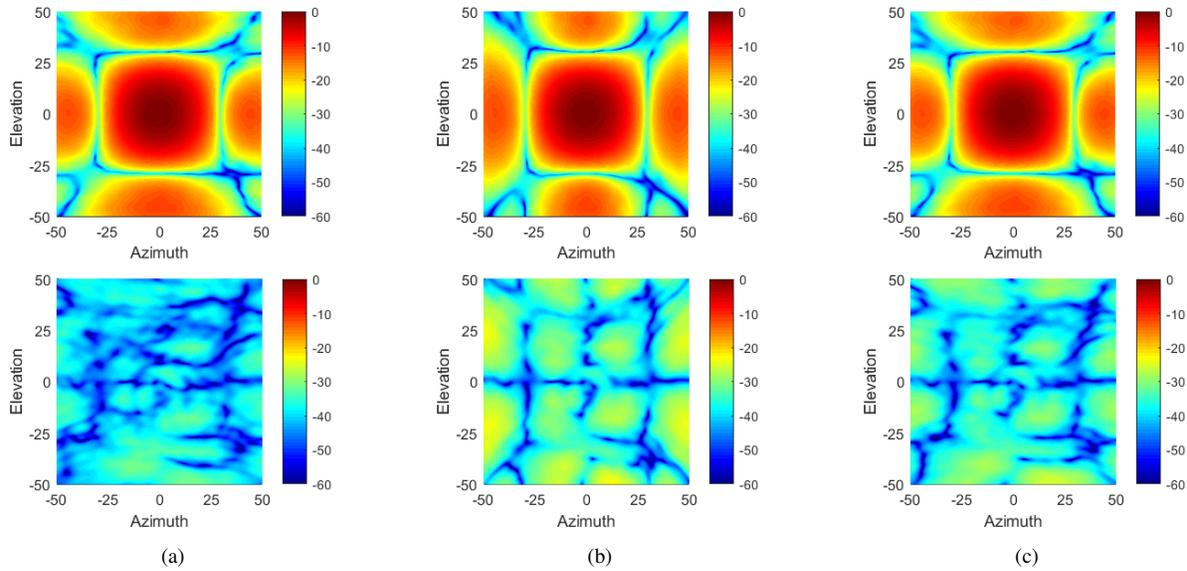
Fig. 18: Measured polarimetric 4x4 planar phased array radiation patterns with H-polarization at broadside; co- and cross-polarization magnitude in dB according to (a) Ludwig 2-I, (b) Ludwig 2-II (second row), and (c) Ludwig 3.
