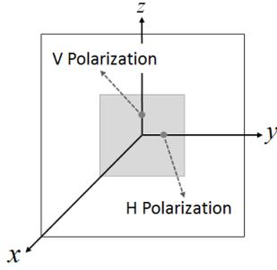
Fig. 3: Dual-polarized antenna element in the  $y$ - $z$  plane.
