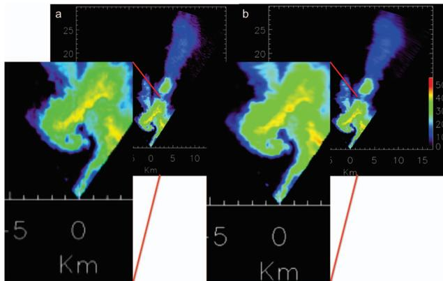
Fig. 7. a: Ground truth reflectivity as seen by X-POL of a supercell on May 13th, 2009 near Woodward, OK. b: Resultant reflectivity fields from the simulated phase-tilt antenna system.
