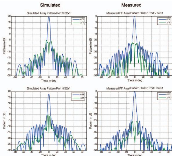
**Fig. 2.** Passive array antenna elevation patterns, simulated and measured, for co- and cross-polarization in horizontal and vertical planes
