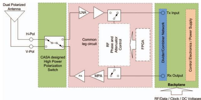
**Fig. 3.** Block diagram of the T/R module component
