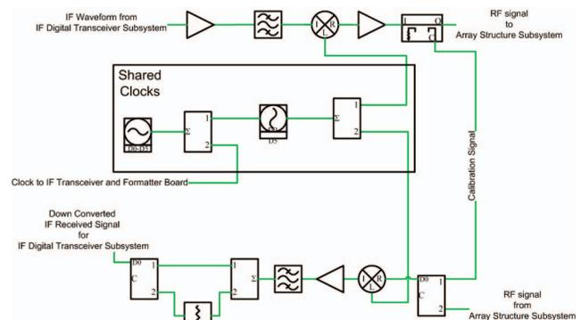
**Fig. 6.** Block diagram of Up/Down Conversion Subsystem
