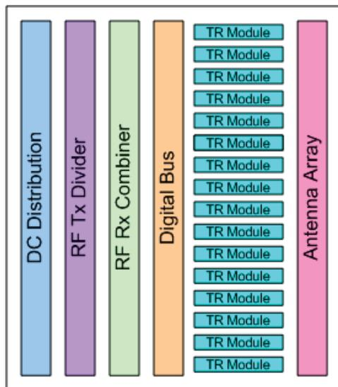
**Fig. 4.** Block diagram of the LRU and backplane component
