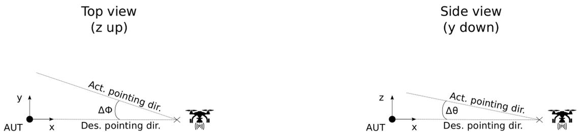
Figure 3.16: Illustration of the gimbal drift effect on the antenna pattern measurements. The probe mounted on the UAV excites the AUT—or receive its signal—at different angles in azimuth and elevation.  $\Delta\Phi$  and  $\Delta\theta$  correspond to these errors respectively.
