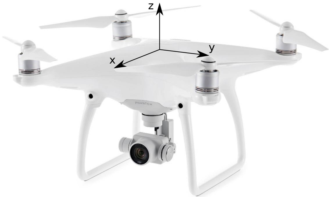
Figure 4.1: The arrangement used for the dynamical model of the quadcopter, illustrated on a DJI Phantom UAV.
