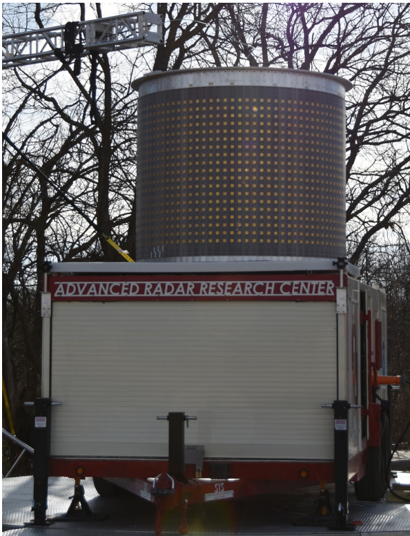
Fig. 1. OU/NSSL CPPAR demonstrator on turntable at far-field test site.
