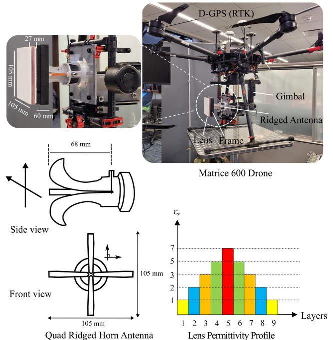
Fig. 1: Illustration of the drone model carrying the ridged horn antenna with the proposed lens prototype.
