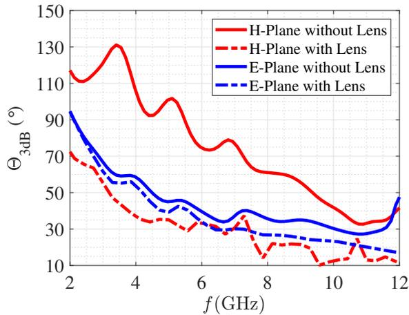
Fig. 2: Simulated 3dB beamwidth comparison in the principle planes of the proposed ridged horn antenna with and without the proposed lens structure.
