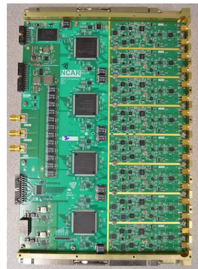
Figure 7. Picture of a brick module composed by 8x1 ATAR T/R modules based on COTS components.
