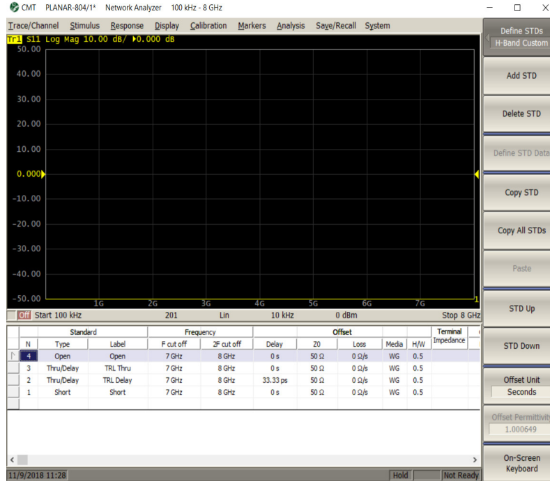
Figure 4.22: Testing: S2VNA calibration kit.
