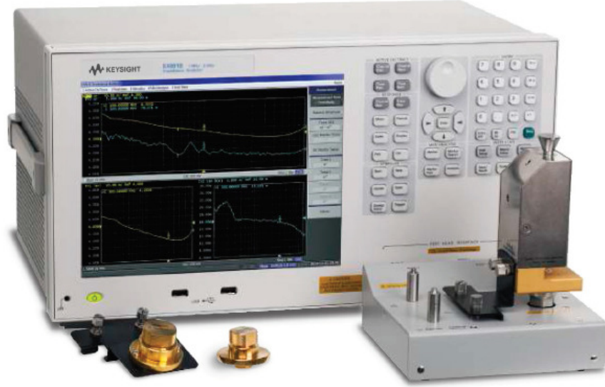
Figure 3.2: Test setup for measuring the admittance of a material [1].
