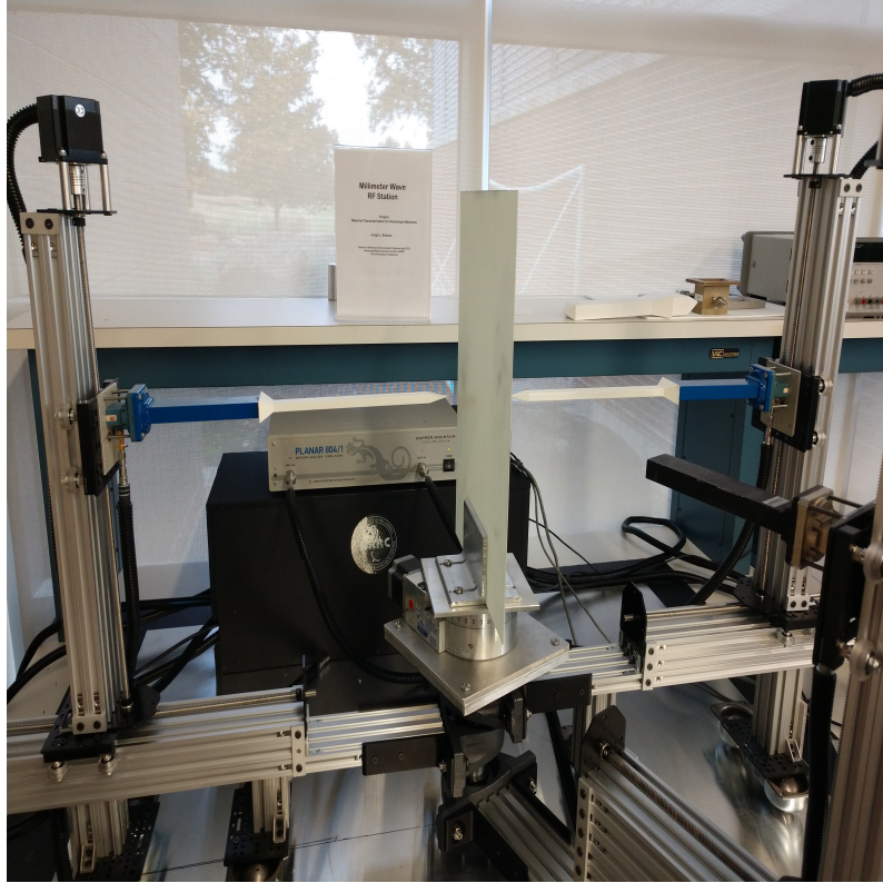
Figure 4.24: Testing: normal incidence measurement.
