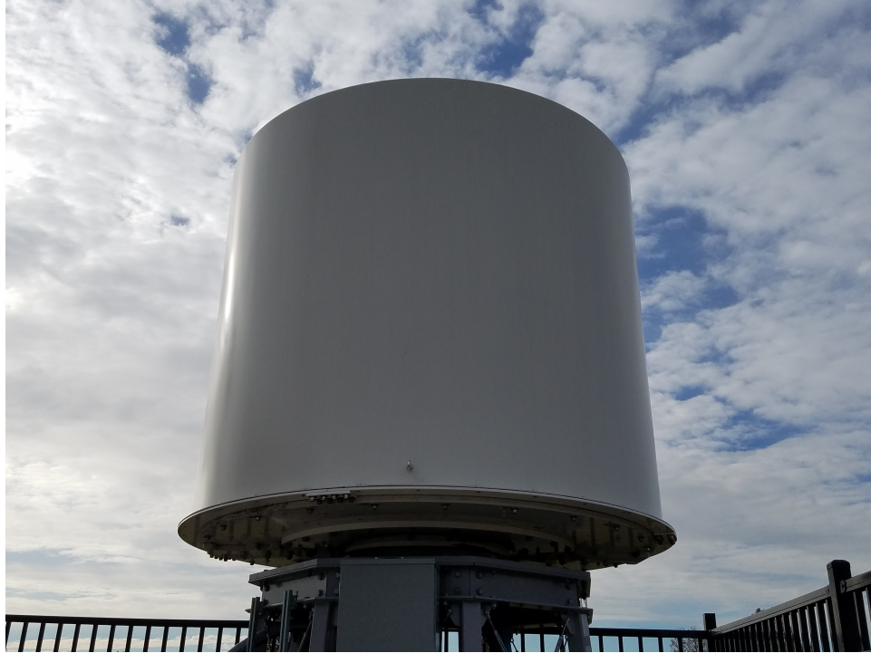
Figure 2.8: A photograph of the S-band cylindrical radome of the CPPAR (Fulton et al. 2017).
