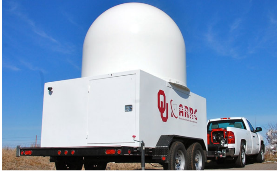
Figure 2.7: The X-band bullet shape radome of the X-band PX-1000 (Cheong et al. 2013). The radome stackup is A-sandwich type with honeycomb as a core. Photo source: https://onenet.net/onenets-high-speed-capabilities-support-advanced-radar-research-in-oklahoma/ .
