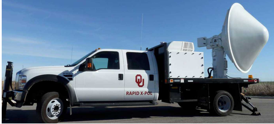
Figure 2.6: The X-band partial radome of the RaXPol (Pazmany et al. 2013). This radome is designed with the monolithic-wall topology which belongs to the category of thin skin. Photo source https://arrc.ou.edu/radars.html .
