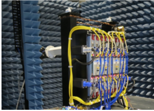
Fig. 3: Near-field panel measurement set-up. Eight OctoBlades are installed in one panel. Here, the orifice of the probe is facing the panel's aperture.
