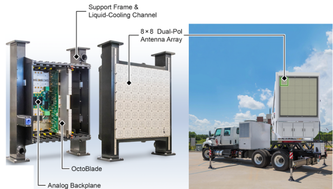
Fig. 1: On the left an 8 x 8 element array panel, on the right the full array of 32x32 elements on an S-Band Mobile Radar.
