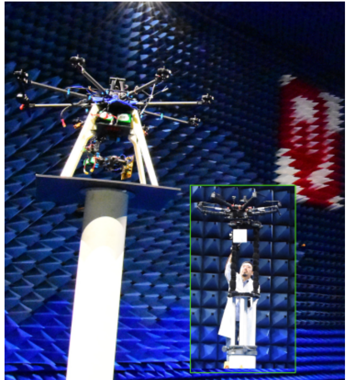
Fig. 1. ARRC UASs units for S-band antenna pattern and radar system characterization. In the left, an octocopter, and in the right, an hexacopter platform during RF test of the antenna array transmitter probe in the far-field range at the Radar Innovations Laboratory (RIL) at The University of Oklahoma.
