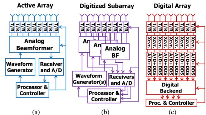
Fig. 1: Three generic beamforming architectures with digitization [10].
