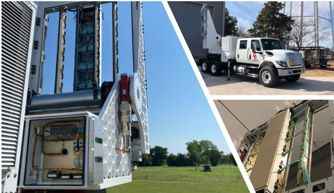
Fig. 1. Horus all-digital PAR during integration (partial array only) and initial field deployments.
