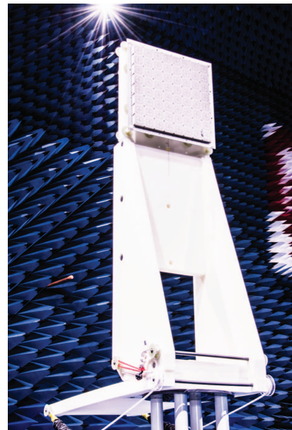
Fig. 5: Antenna fixture in the ARRC's far-field chamber at The University of Oklahoma to measure the 8x8 array.
