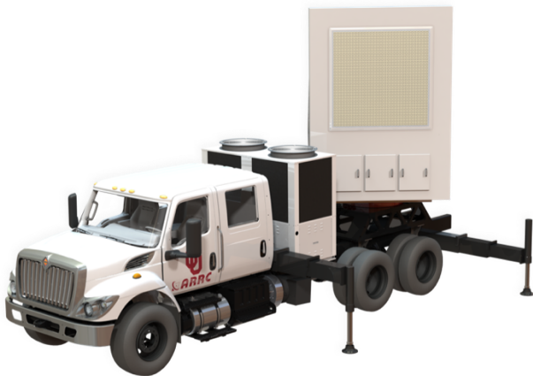
Fig. 2: Mobile S-Band, Dual-Pol, Digital-at-Every-Element Radar [13].
