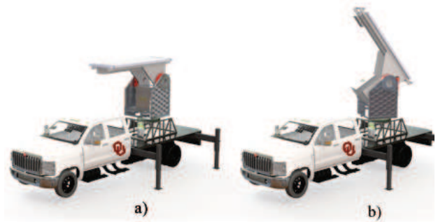
Fig. 4. Rendering of the KaRVIR trucks for field deployment. a) Vertical pointing and transportation mode. b) Scanning operation mode.
