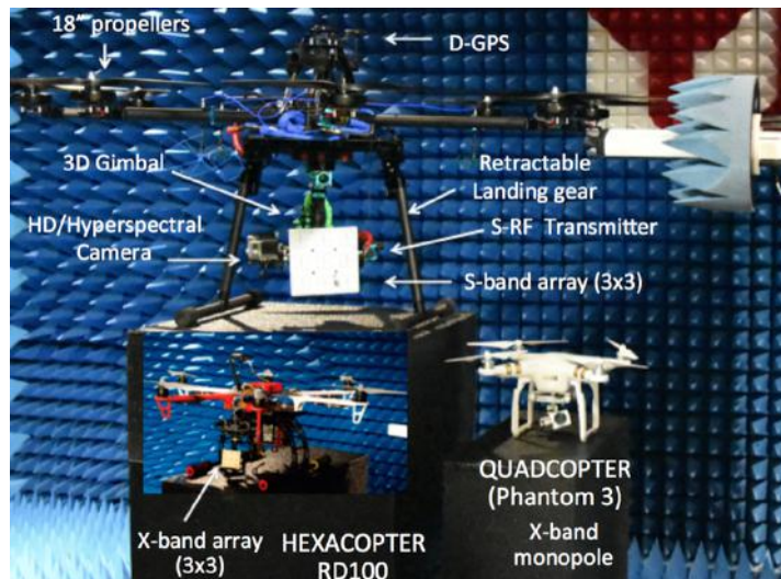
Fig. 4. OU UAS’ platforms used for antenna characterization and radar calibration. On the left, the Intelinair RD100 platform with an X-band 4x4 dual polarized array antenna. In the middle, the OU UAVRF1250 with an S-band array of 3x3 elements. On the right, the Phantom 3 with a one-quarter-wavelength X-band monopole antenna
