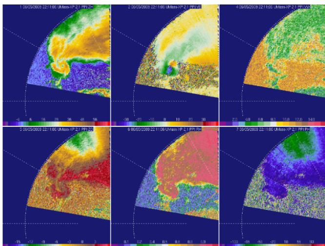
Fig. 4. Left to right from upper left: Reflectivity, Doppler velocity, Doppler spectrum width, Differential Reflectivity, Polarization correlation coefficient, and Differential Phase observations of the Goshen County tornado.
