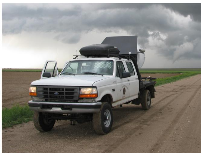
Fig. 1. The UMass W-band mobile Doppler radar on May 25, 2010 near Tribune, KS. Tornado is visible in distance. photo (c) R. Tanamachi.
