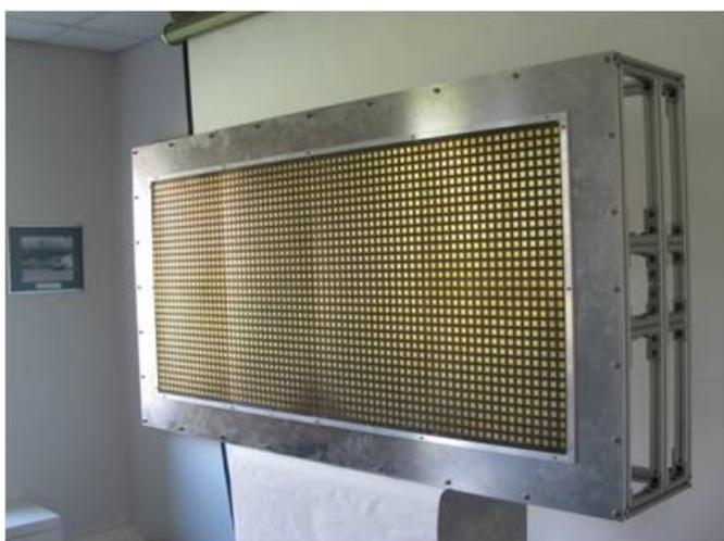
Fig. 5. The radiating face of the CASA "Phase-tilt" dual-polarized phased-array. The array consists of four modules of 16 elements comprised of series-fed aperture-coupled microstrip patches.
