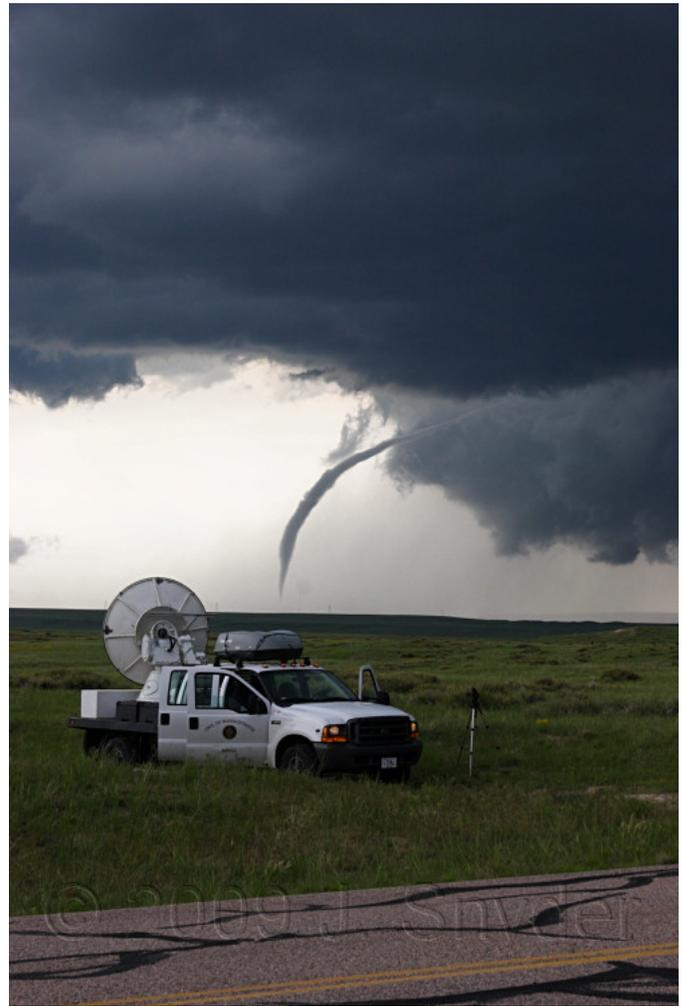
Fig. 3. The UMass X-Pol mobile Doppler radar and the decaying Goshen County WY tornado observed on 5 June 2009. photo (c) J. Snyder.
