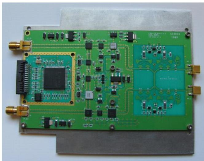
Fig. 6. A T/R module developed for the CASA solid-state X-band dual-polarized phased-array. Transceiver ports are on the left, antenna ports are on the right.
